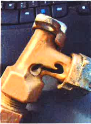
The damaged curb-stop
